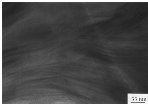
FIG. 2. Transmission electron micrograph of ESO/EPON ® 828/organo-clay composites. EPON ® 828 furnished by Shell Chemical (Houston, TX). For abbreviation see Figure 1.
